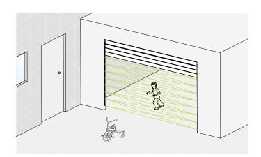
CEDES offers a wide range of products that allow safeguarding of residential garage doors in a cost competitive way. Key advantage, using optical sensors, is that any physical contact between the door and the persons/objects is prevented. This increases safety and comfort for people and prolongs the life span of the installed door. CEDES products are well proven in the industry and have, depending on the type, a TÜV safety certification.
