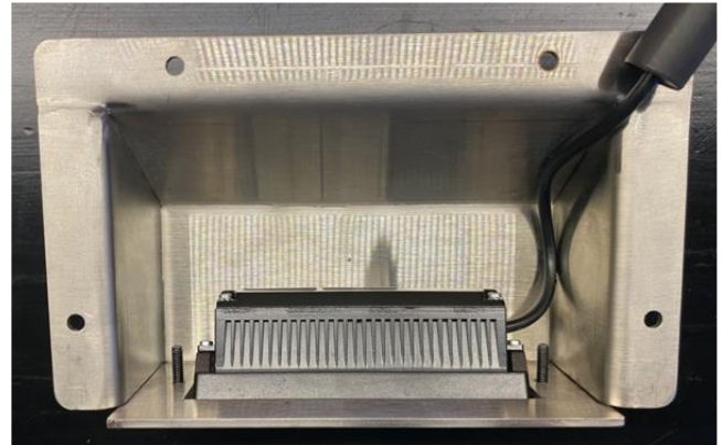
Figure 38: CabSafe 3D Sensor installed in back of transom bracket
