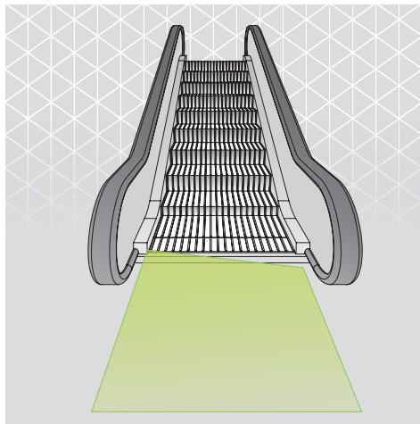
**Figure 1:** TOF/Start detects intending passengers approaching an escalator.
