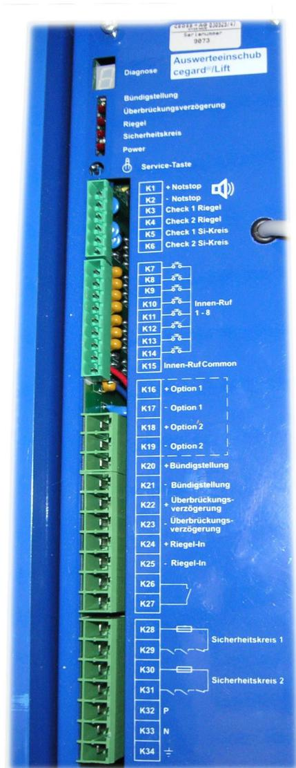
Figure 10: Connection terminals plug-in system controller
