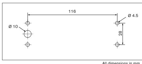
**Figure 8:** Backside view of a surface-mounted TPS
