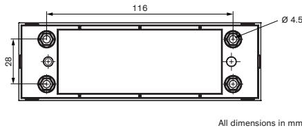
**Figure 7:** Backside view of a flush-mounted TPS
