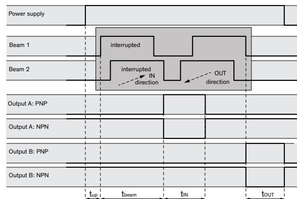
If an object passes through both beams in IN or OUT direction, an output pulse is sent to the corresponding output.
