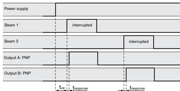
Upon interruption of either light beam, the corresponding PNP output is switched to HIGH.
